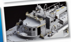
This 1:72 scale naval ship has extra detail added. The gold-colored components are made of brass.
